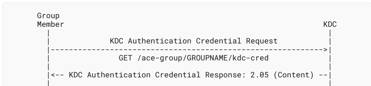
Figure 21: Message Flow of KDC Authentication Credential Request-Response to Obtain the Authentication Credential of the KDC
